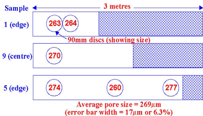
Figure 7: Effect of sample position on aperture size
