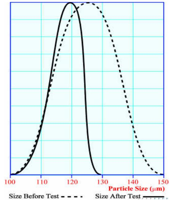
Figure 6: Particle size difference in microspheres after passing test mesh
