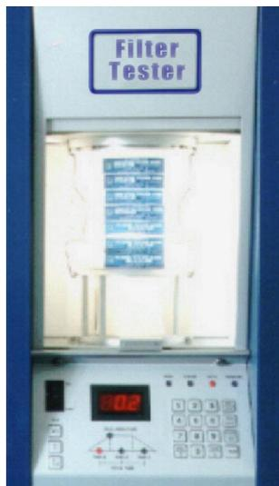
**figure 3: The sonic filter tester (Gilsonic)**
