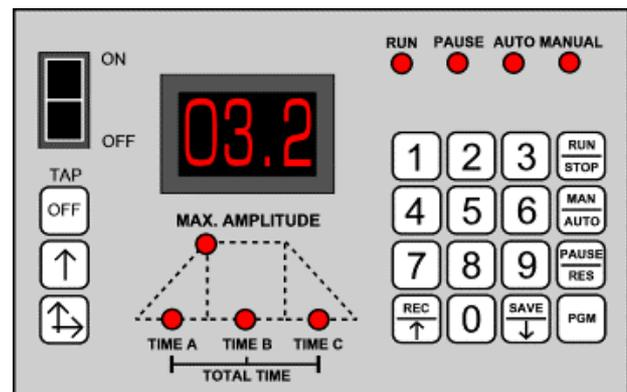
**figure 5: Gilsonic AutoSiever control panel**
