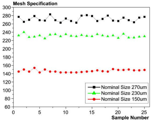
**Figure 8: Size variations of sand screen meshes using the sonic testing method**
