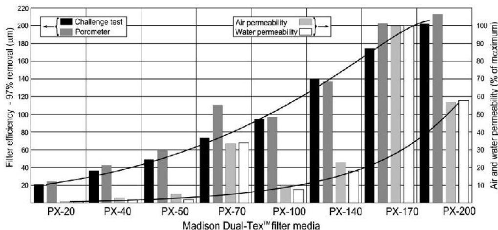
**Figure 11.** Comparison of test methods on a range of Dual-Text™ filter media
