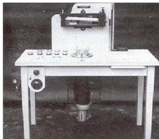
**Figure 10.** Frazier low pressure machine for measuring air permeability
