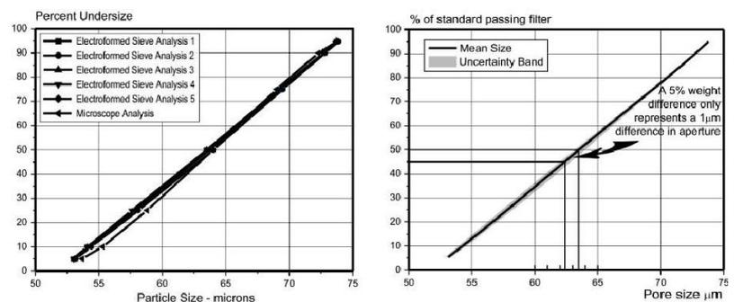
**Figure 5.** Construction of filter standard calibration graph
