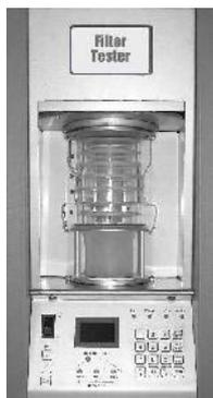
**Figure 6.** A filter challenge tester based on the Gilson sonic autosifter
