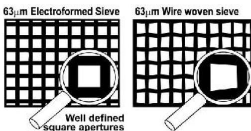
**Figure 4.** Electroformed sieve have well defined accurate apertures
