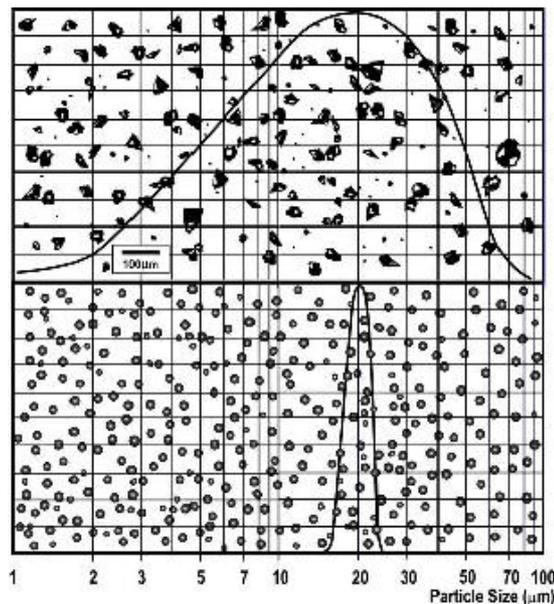
**Figure 3.** A test dust compared to narrow distribution spherical test standard
